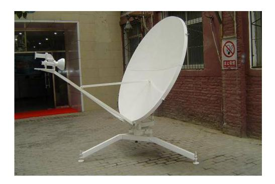
The Ruman tech lightweight 1.8m flyaway antenna is designed for transmit and receive in C/Ku band. The portable antenna consist of composite reflectors and tripod base mount. Repeatability maintained with precision registration of the 4-piece reflector segments and support structure. The complete 1.8meter antenna system is packaged in two portable box or two bags.
